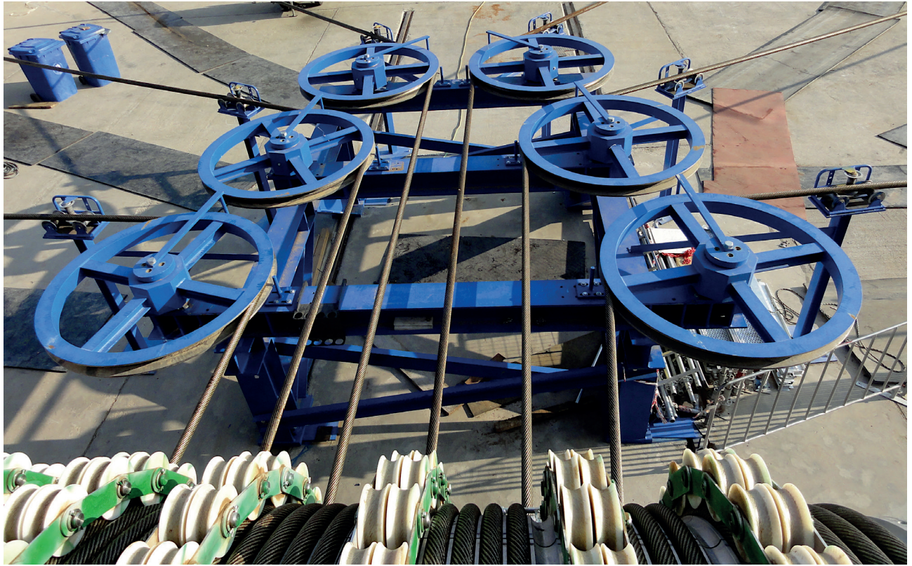
View from the mobile friction winch onto the horizontal deflector sheaves with incoming ropes.
