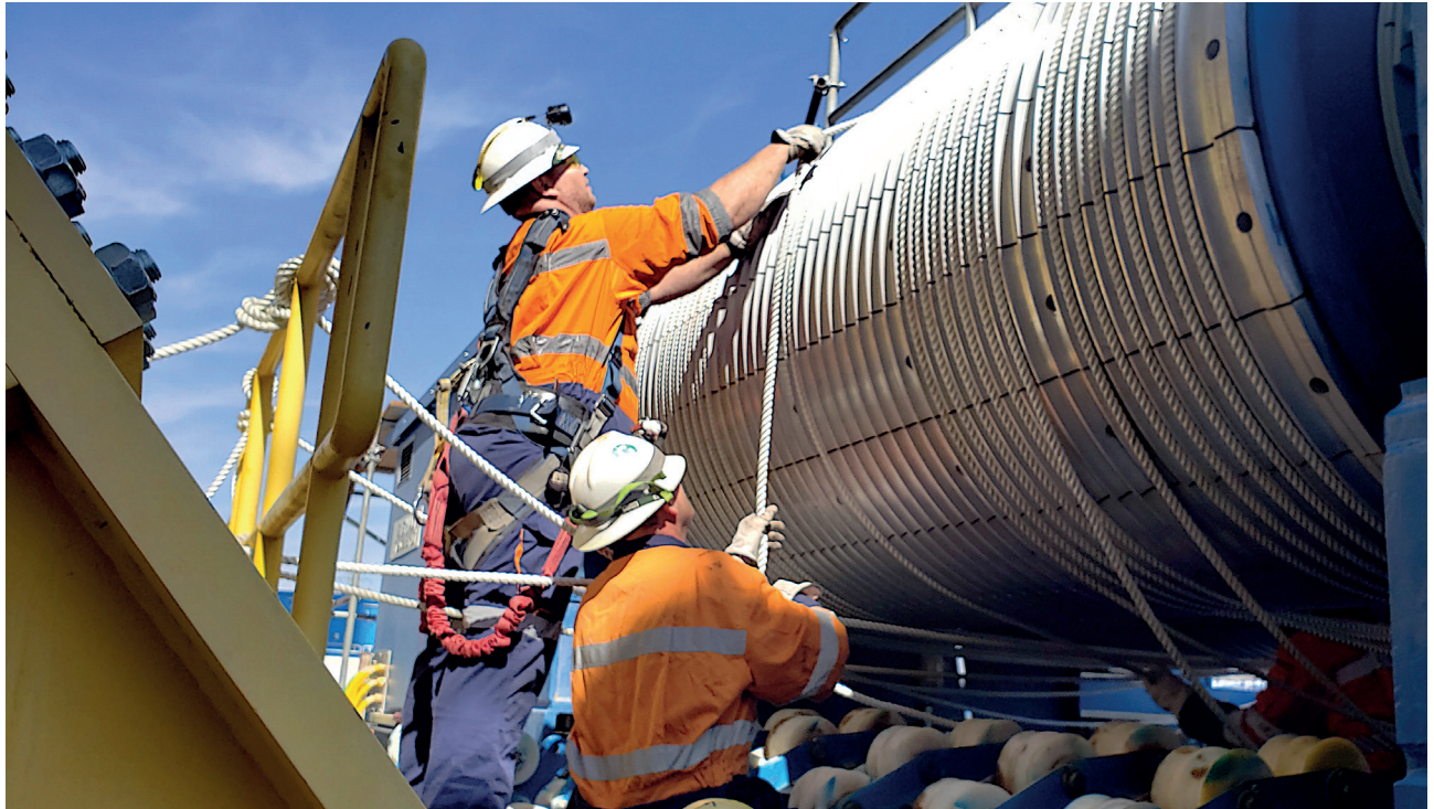
Employees of the service team while working on the mobile friction winch.
