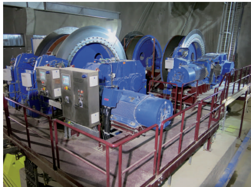
Fig. 8: View of the shaft hoisting systems for Lot D; CS winch in front; IPF at the rear
